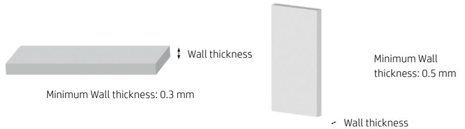
For parts with a high aspect ratio, you are recommended to increase the wall thickness, or add ribs or fillets to reinforce the part.
